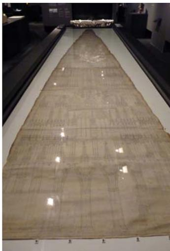
These are the original drawings for the north tower made on six separate parchments (calf hides) six metres in length and completed in 1464. The tower reached only 68 metres before work stopped, never to be resumed. I took this photo before being told "no photos" and I'm glad I did because the
